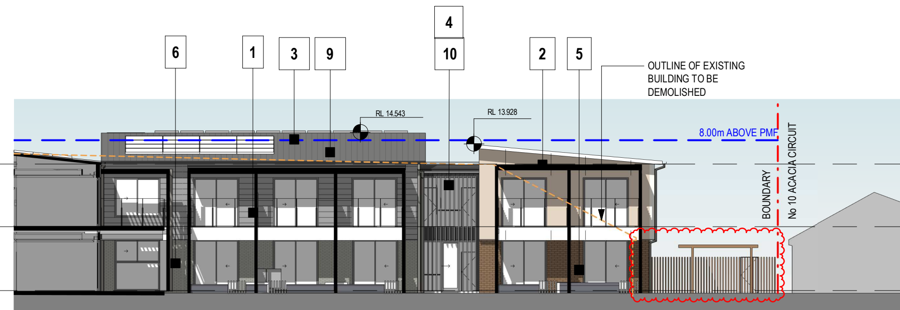
5 DA - ELEVATION - COURTYARD 5 - WING 4 1:200
